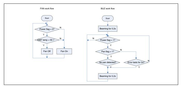
Figure 3-4 Fan and BUZ Workflow
